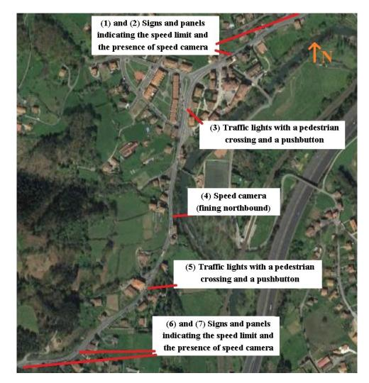
Figure 4. Locations of the traffic calming measures and other elements in Arrankudiaga (Spain).
