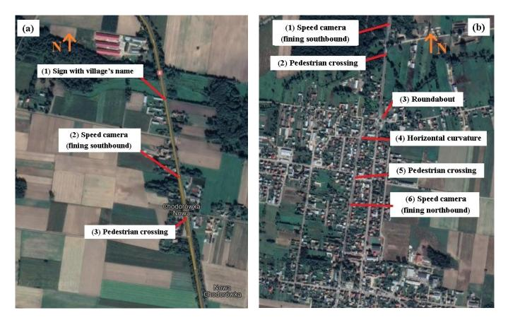
Figure 3. Locations of the traffic calming measures and other elements in (a) Chodorówka Nowa; (b) Suchowola.
