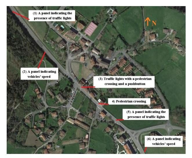
Figure 5. Locations of the traffic calming measures and other elements in Arrespalditza/Respaldiza (Spain).
