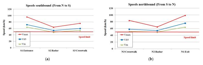
Figure 6. Speed at each controlled point in Chodorówka Nowa (Poland): (a) southbound, (b) northbound.
