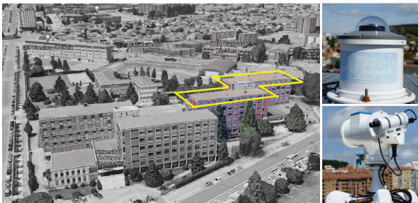
FIGURE 4: Location of the experimental equipment on the roof of the Higher Polytechnic School building at the University of Burgos with the SONA 201-D sky camera (top) and EKO MS-321LR (bottom) (source: Google Earth).
