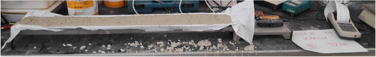
Figure 8. Arrangement of setting shrinkage test.
