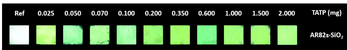
Figure S61. Response of AR82s-SiO 2 exposed to different quantities of TATP.
