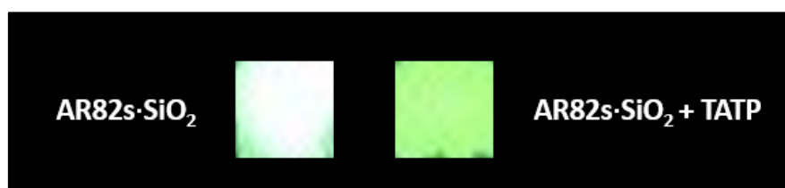
Figure S57. Color comparison between the nanoparticles with the probe over glass plates before and after the exposure to TATP.
