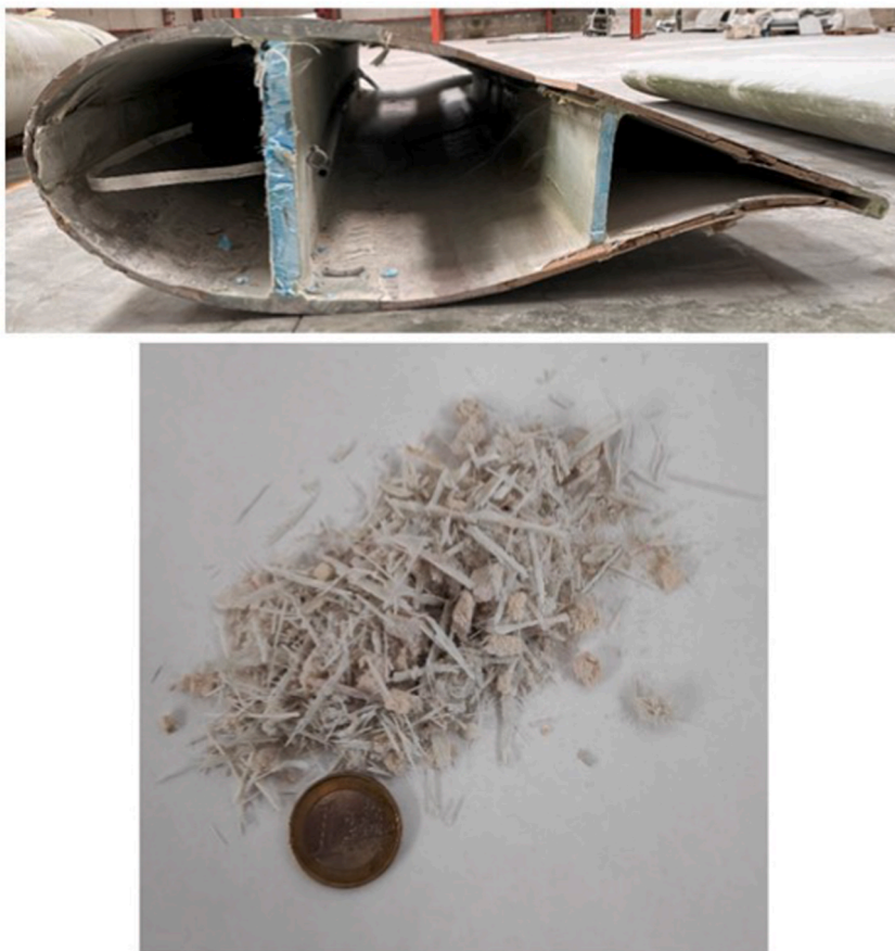
Fig. 2. Transverse section of a wind-turbine blade (up) and raw-crushed wind-turbine blade (down).
