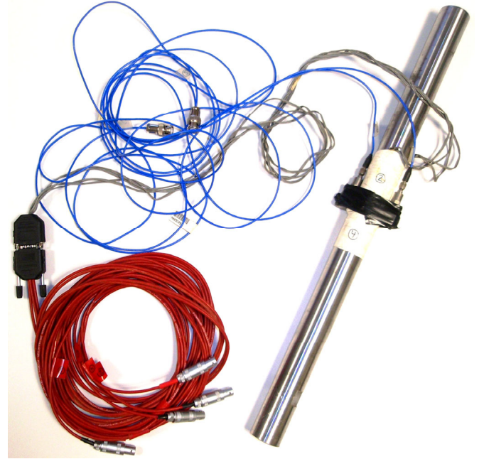
Figure 1. Instrumented portion of the rod string with the strain gauges and the accelerometers.
