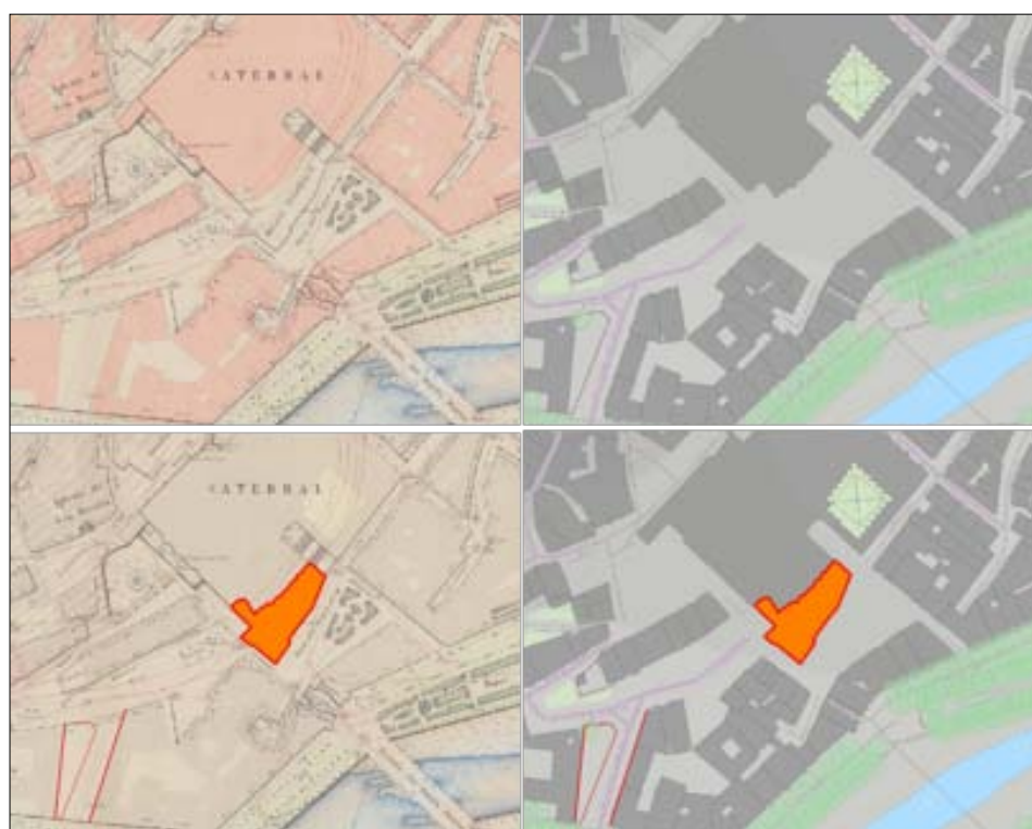
Figure 5: Conversion of a disappeared old building into a vector. Geometrical identification, measurement of surfaces, and integration into present cartography
