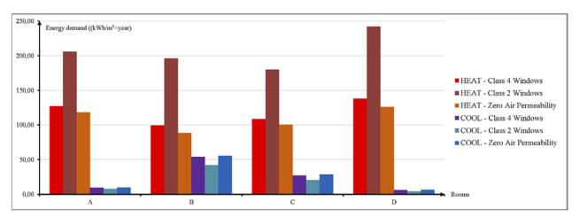
Fig. 6. Results of the energy simulations related with the windows air permeability.
