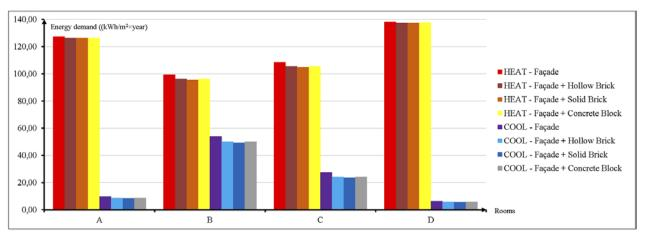
Fig.7. Results of the energy simulations related with the façades thermal inertia.
