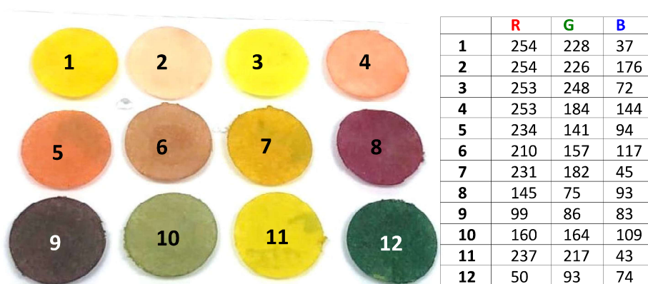
Figure 3. (Left) Filter paper discs coated with sensory polymers after spraying an acid solution of sodium nitrite (0.1 g \text{NaNO}_2 , 25 mL water, 2.5 mL HCl 37%) and an aqueous solution of NaOH (1M). (Right) RGB color definition parameters for each disc.
