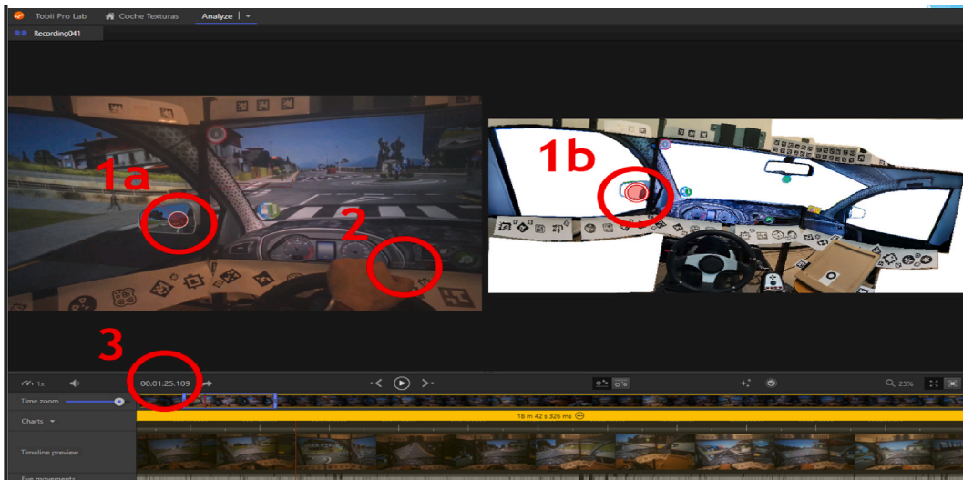
Fig. 3. (1a) eye fixation in a video recorded by the eye tracker; (1b) position around the vehicle’s cockpit as detected by the Tobii Pro Lab software, in this case, the left mirror; (2) timestamp within the simulator that enables the synchronization with the eye tracker timestamp; (3) eye tracker timestamp that allows computing the difference between both systems.
